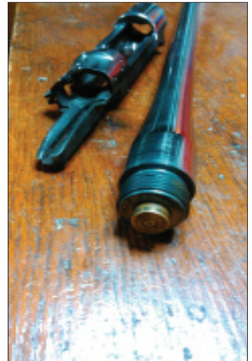
This shows the chambered and threaded barrel.
