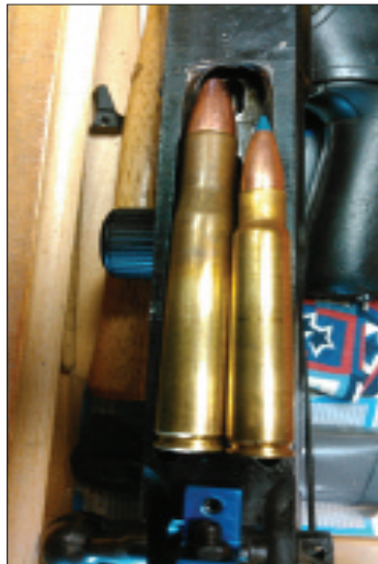
The difference in the 8x57 Mauser and the 404 Jeffery shows how much the action was opened up.
