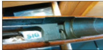
Here is the glass-bedded stock showing the integral magazine box front.
