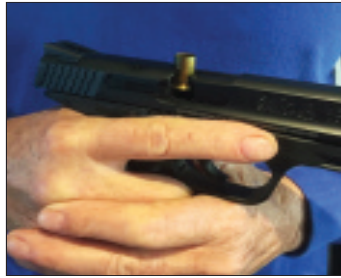
A stovepipe occurs when a shell doesn't get clear before the slide comes forward.
