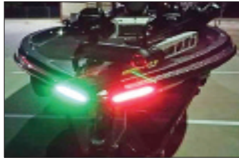
NOT SAFE – Navigation lights like these don't pass muster and don't make for safe boating.
