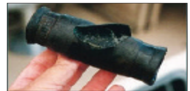
Cracked Fuel Line
